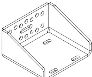
Pre drilled Plates (suit MAN, Volvo & Scania chassis with 14mm holes & Mercedes chassis with 16mm holes (**holes need to be drilled out to 16.5mm**)
