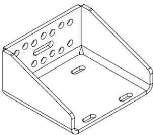
Pre drilled Plates (suit MAN, Volvo & Scania chassis with 14mm holes & Mercedes chassis with 16mm holes **(holes need to be drilled out to 16.5mm)**
